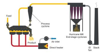
**ReCyclone® MH** convertible to a ReCyclone® EH for fertilizer dust emission control under 50mg/Nm³ after a double tunnel dryer.
