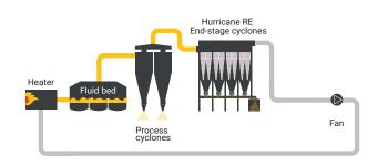
**Hurricane HRbH** high efficiency process cyclones with alumina tile to maximize the recovery of lithium hydroxide particles after a Spray Dryer.
