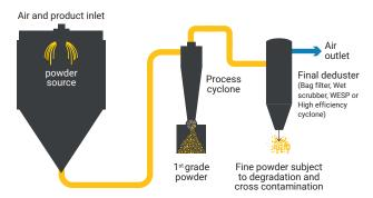
Generally, a **process cyclone** serves the purpose of separating the main fraction of 1<sup>st</sup> **grade powder** and a **final deduster** avoids the fines to escape to the atmosphere. Depending on how sensitive the powder is and on the process characteristics (e.g. product rotation), fines may or not be considered as waste due to the limitations of the final deduster.
