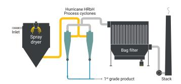
**Hurricane MK** cyclones to increase the collection of sulphanilic acid fines escaping the process cyclone after a fluidized bed dryer to meet emissions of  $\sim 50 \text{ mg/Nm}^3$ .
