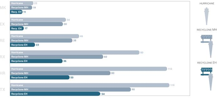
$Residual\ emissions\ (mg/Nm^3)\ at\ the\ stack\ from\ page\ 5.\ Example:\ Fluidized\ Bed\ Drying\ of\ Sulphanilic\ Acid$
