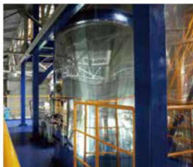
Atomization mode: Rotary atomizer Drying chamber diameter: \phi 3400 mm Water evaporation capacity: 86 kg/h
